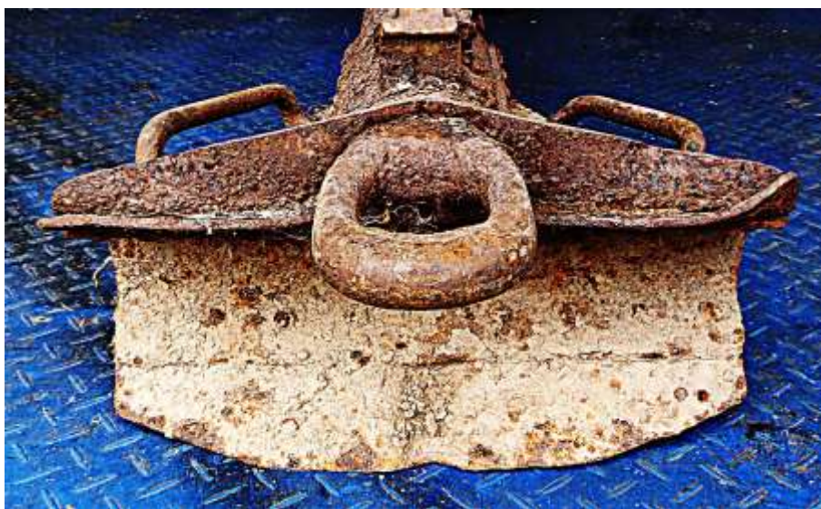
Figure 11 the end of the trail and towing eye.
