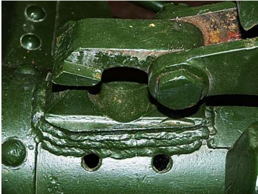
Figure 14 close up of a lever fitting welded back in place leaving the rivet holes open
