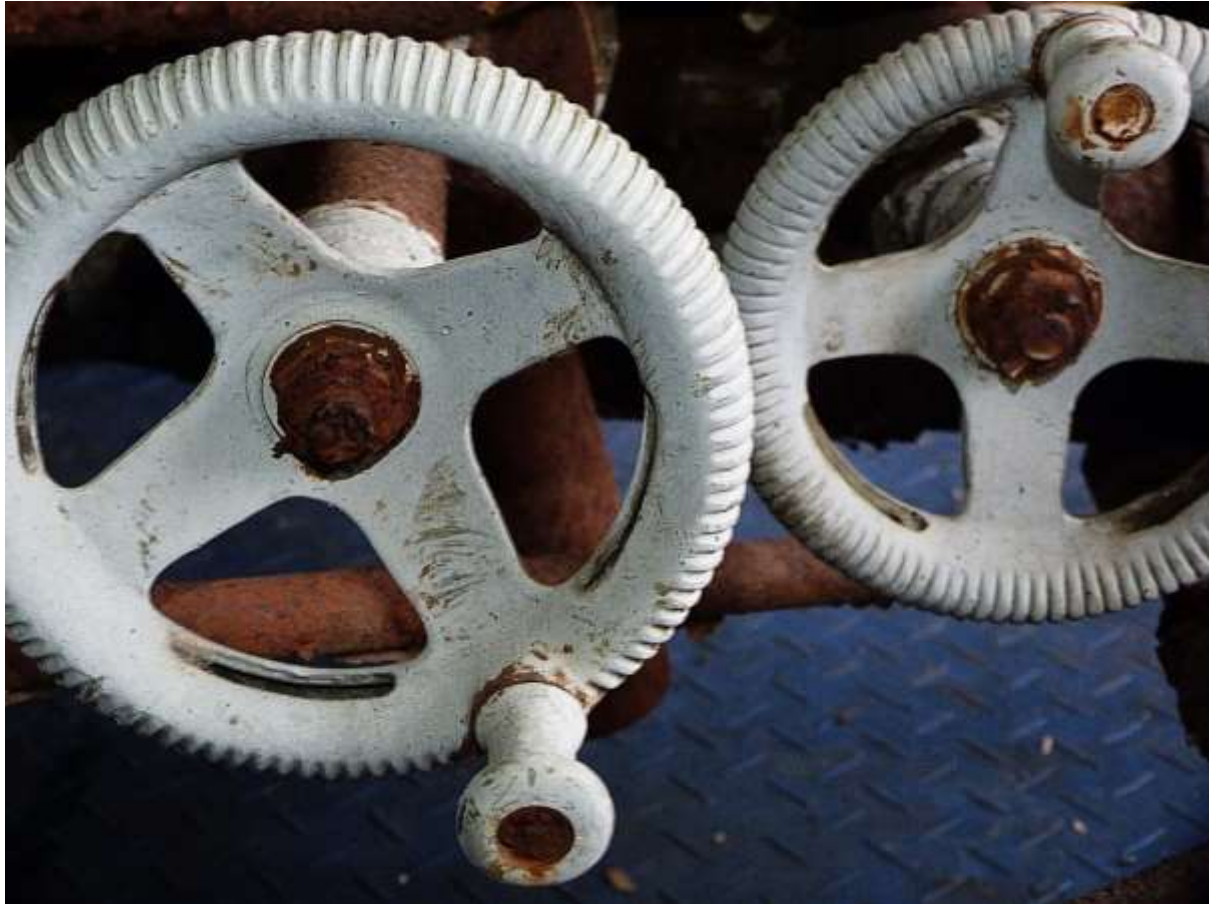
Figure 18 the hand wheels for the elevating and traversing mechanism
